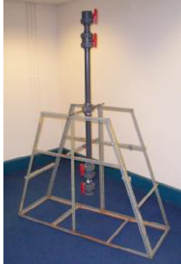
Figure 4 Settling Column Apparatus for Effluent Characterisation
